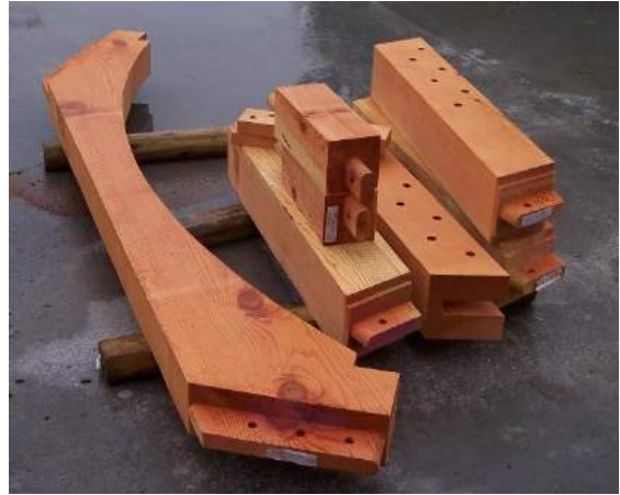
CNC fabricated timbers
