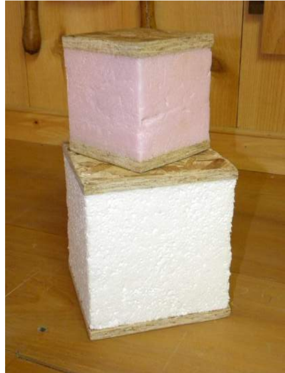
SIPs with XPS core (pink) and EPS core (white)
